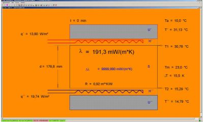
With end of measurement the program automatically prints the test report, which is an important request of **EN12667:2001**; additional test declarations for this report will be insert in remanent text-fields. **WinHLT#** stores all these data as a dataset in a table-file on the hard-disc also.
