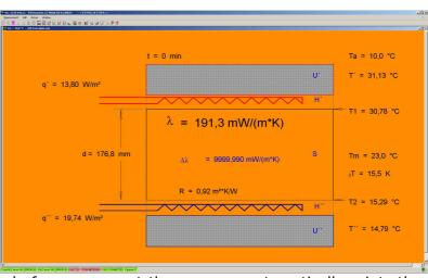
With end of measurement the program automatically prints the test report, which is an important request of **EN12667:2001**; additional test declarations for this report will be insert in remanent text-fields. **WinHLT#** stores all these data as a data-set in a table-file on the hard-disc also.
