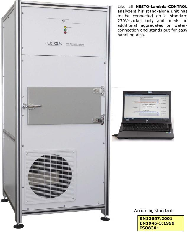
the instrument measures the thermal transfer properties under steady-state conditions of
